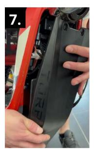
STEP 8: Use the longer M6 screws and a larger hex key to fasten the shield to the frame.
