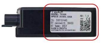
On the side of each Torp controller box and on the controller itself, you'll find a silver sticker displaying essential identification details: Serial Number, Bluetooth Password, Bluetooth Name, Model, and Hardware Version. You'll need the Bluetooth password and Bluetooth name to connect your controller to the Torp App, and the serial number to access support from the Torp team. Please ensure that you do not remove the sticker from the controller, and keep this information securely stored.
