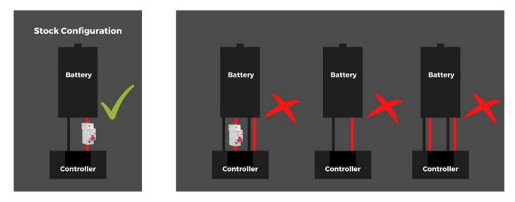
Use only tools and screws that came with the controller. Using the tools and screws that were not included in the parcel, not following these instructions, or not using the circuit breaker, can cause serious damage to you and your bike and voids your 2-year warranty.
